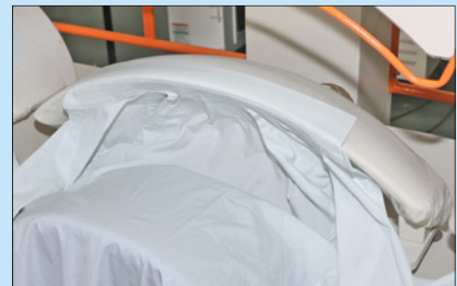
四曲面斜角立體領模 Four-curve-surfaced & oblique-angled 3D collar mould
