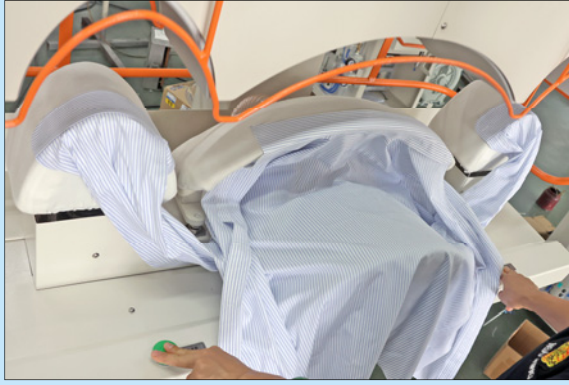
領袖壓熨操作一 Collar & cuff pressing operation #1
