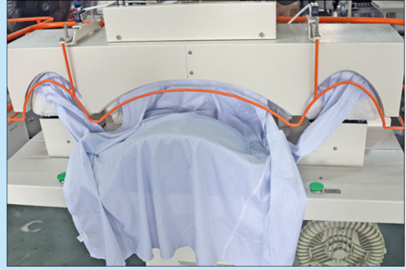
領袖壓熨操作二 Collar & cuff pressing operation #2
