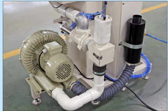
獨立真空抽濕系統 Independent vacuum pump system
