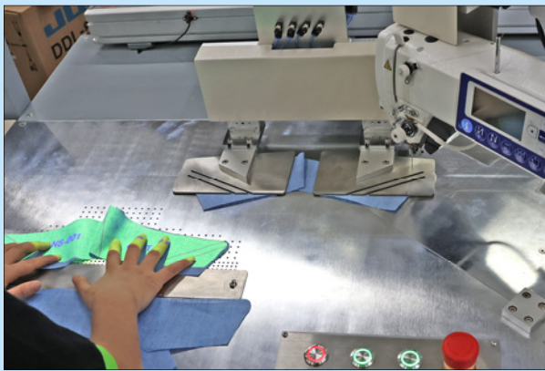
雙工位設計，可同時鋪料和車縫 Twin stations design for simultaneous operation of material placement and sewing
